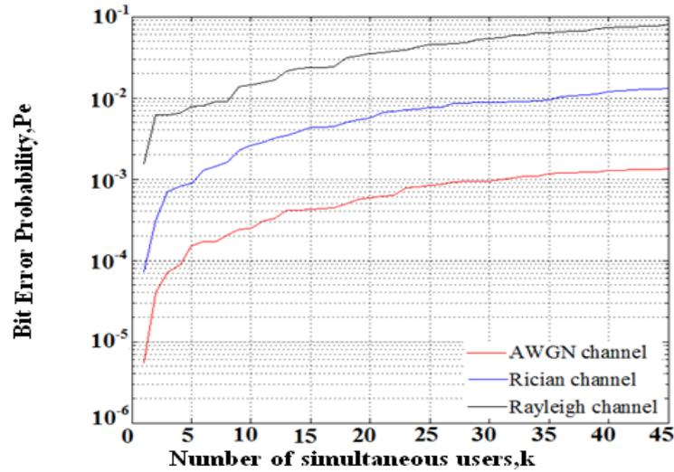
Fig. 4. BEPs of the chaotic/FH-CDMA scheme versus the number of simultaneous users K over AWGN, Rician and Rayleigh fading channels
