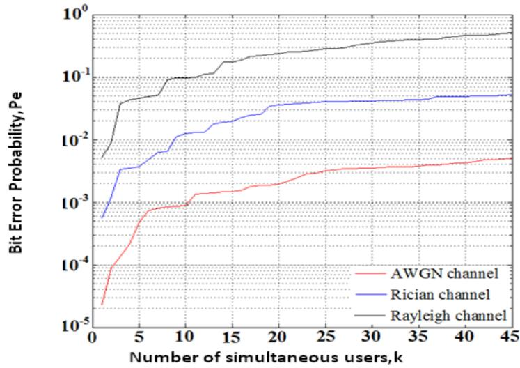
Fig. 3. BEPs of the prime/FH-CDMA scheme versus the number of simultaneous users K over AWGN, Rician and Rayleigh fading channels.
