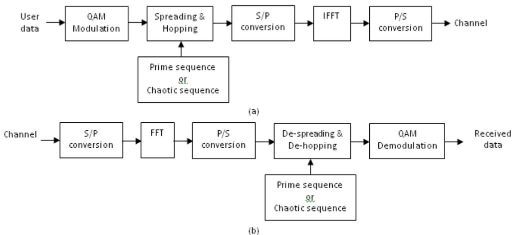
Fig 2: Block diagram representation of (a) Transmitter and (b) Receiver
