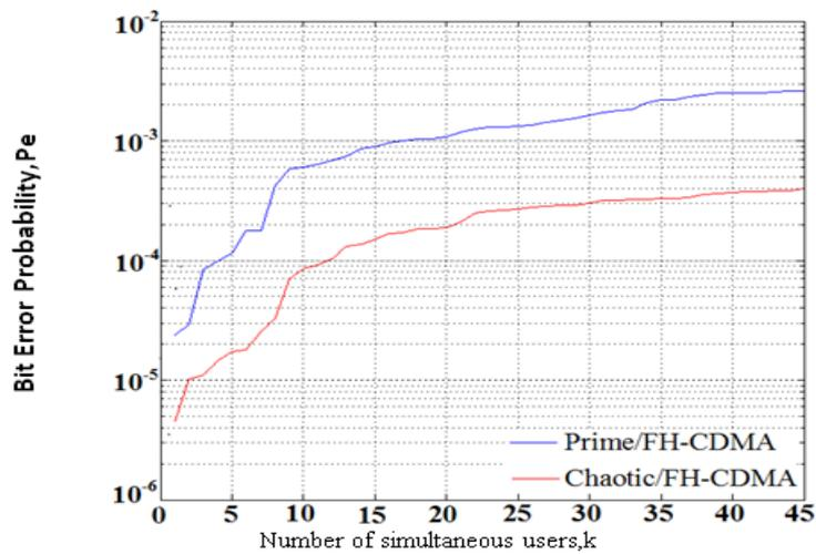
Fig. 5. BEPs comparison of chaotic/FH-CDMA and prime/FH-CDMA schemes versus number of simultaneous users K over AWGN channel.
