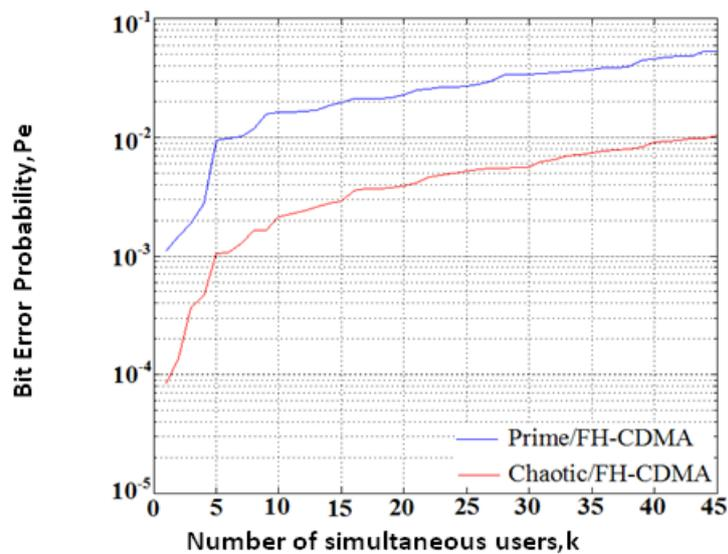
Fig. 6. BEPs comparison of chaotic/ FH-CDMA and prime/FH-CDMA schemes versus number of simultaneous users K over Rician fading channel.
